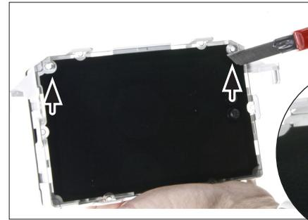
6. Remove OEM display. Cut away overlapping pins left and right
