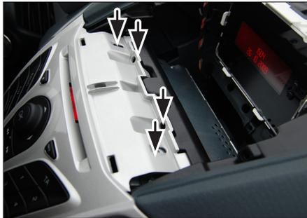
3. Remove the 4 screws of the OEM head unit
