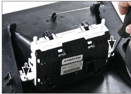
9. Fix OEM display with 2 screws
